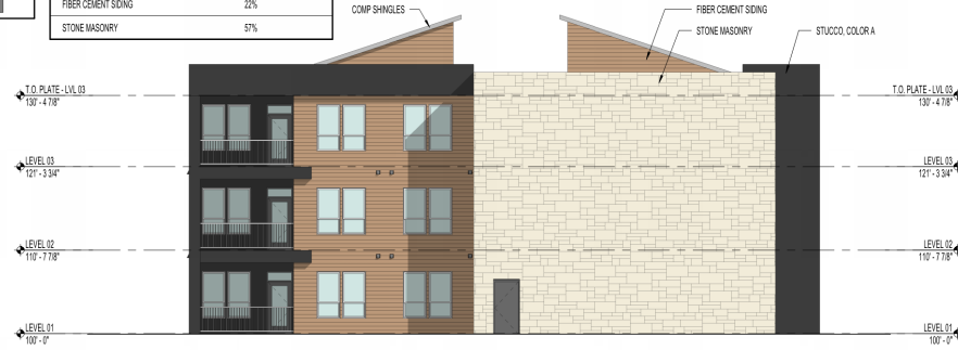
3 TYPE VI (BLDG #9) - SIDE ELEVATION (AREA A) 1/8" = 1'-0"
